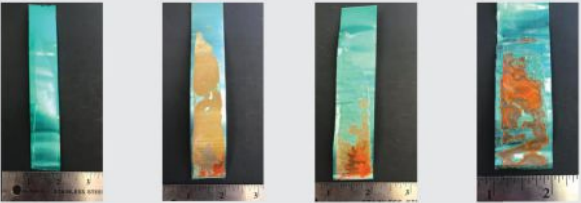
Figure 13 - LLFlex, Sample A, Sample B, and Sample C After Immersion in Acetic Acid
