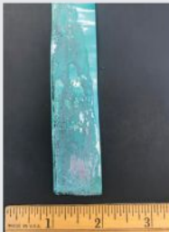
Figure 6 - Sample B Exhibiting Cohesive Failure
