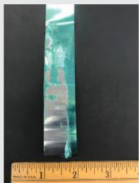
Figure 7 - Sample C Exhibiting Metal Failure
